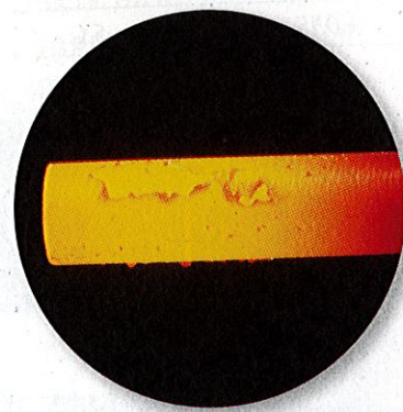
At about 1,200 °C, the metal glows yellow.
