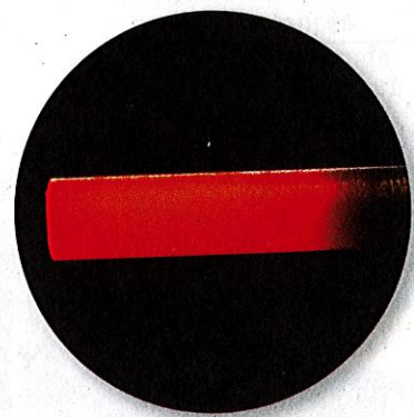
A steel bar glows red when heated to about 600 °C.
